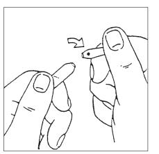
Coloured dot upwards Break off top of ampoule in a downward direction.
