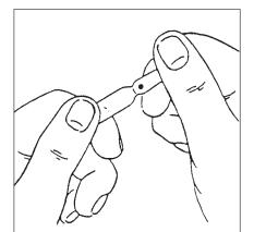
**Coloured dot upwards** Allow any solution in top of ampoule to flow down by tapping or shaking.
