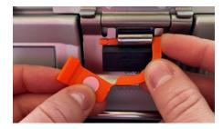
1 Close the latch to secure the lid to the container bottom. Insert the tamper-evident seal through the channel.
