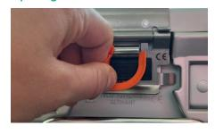
1 Break the seal by simply pulling it away with the finger until it releases.
